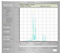
Figure 6 – SignalScope's FFT mode displaying a RTTY signal
