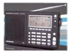
entering frequencies into memory and recalling them was tedious and not well thought out. In order to get to any page of memorized frequencies, one has to hold down the tiny button of that page and scroll through the 10 selections. I like intuitive radios and in this regard, the G5 is not.
