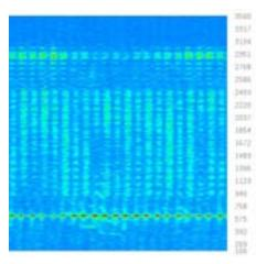
At approximately +605Hz you can note the presence of a distinctive, unmodulated pilot tone which is used by the receiving modem to track frequency errors due to Doppler shift. Then follow 14 tones of 4PSK modulated data, each spaced at 110Hz starting at +935Hz and ending at +2365Hz. Finally, there are two more PSK modulated tones placed around +2915Hz. These are used for synchronization purposes. With that configuration, the system achieves a data rate of 1364bps.
