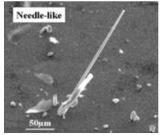
after a product is manufactured. Any soldered component that has a mechanical stress point would be subject to tin whiskers.
